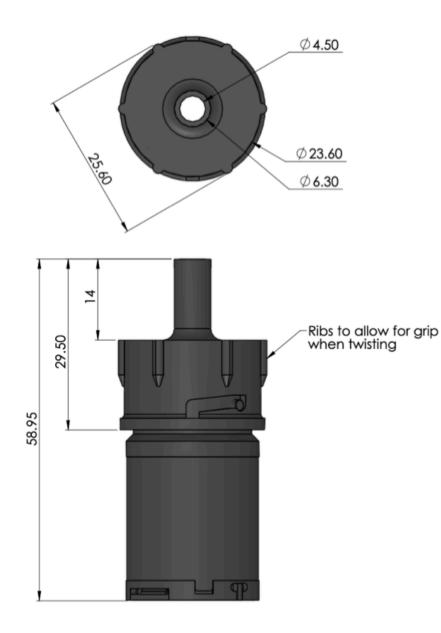
The S+2OX LL sensor can be supplied with a bayonet fit nose adaptor. It is essential to provide a good mechanical seal to face of sensor for accurate trace O2 level measurement. This part is designated S+2OX LLN
