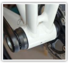
3. Push the left crank with its factory-installed bearing into the left adapter. Align correctly with the right crank and tap into place. NOTE: The wave washer goes between the crank bearing and the left side adapter. Tighten to Campy Ultra-Torque crank to Campagnolo specifications.
