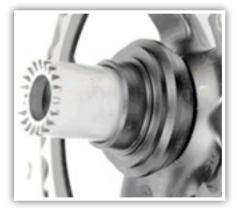
If not already installed, press the PF30 bottom bracket cups into frame. Remove outer dust covers, if present. (Do not remove the bearing seals). Identify left and right side adapters.
