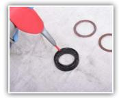
2. Flush out old grease with a de-greaser. Dry bearing to remove any traces of degreaser.
