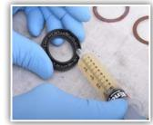
3. Pack bearing with new, clean bearing grease [GR-001].
