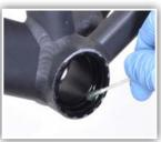
8. Clean and dry bearing bore in cup. Apply thin film of Loctite 603 retaining compound to cup.
