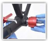
4. Select a sleeve size that has a larger ID than the bearing's OD. Slide receiver cup + reducer sleeve over the rod and up againt cup.
