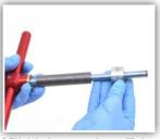
2. Slide the bearing extractor pusher onto a Wheels Mfg Universal BB Press [PRESS-7 or PRESS-7-PRO] rod. Next, add the matching adapter with the tapered end of the adapter opposite the pusher.
