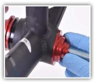
Slide second BB adapter onto threaded rod and into the opposite side of the bottom bracket shell.
