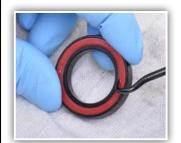
1. Lift up seal using a utility knife or pick. If servicing bearings outside of BB cups, remove both seals. Clean seals and set aside. For Angular Contact bearings, note which side takes the black seal.
