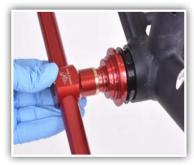
4. Using Wheels Mfg Universal Bottom Bracket Press [PRESS-7 or PRESS-7-PRO], insert one BB adapter into drive side bearing. Match the correct size step on the drift with bearing inner diameter. Slide press handle + rod thru BB adapter and cup.
