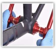
Spin on second press handle and fully tighten until drive side cup is flush with frame.
