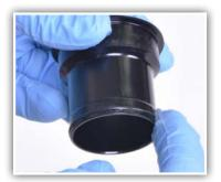
7. Apply a thin layer of grease to the inner o-ring on the male cup.
