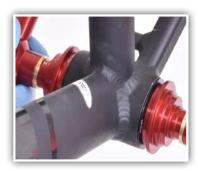
Using Wheels Mfg Universal Bottom Bracket Press [PRESS-7] or PRESS-7-PRO], insert one BB adapter into each bearing. Match the correct size step on the drift with bearing inner diameter. Slide press handle + rod thru BB adapters and cups.
