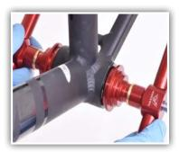
10. Spin on second press hande and fully tighten until non-drive side cup is flush with frame.
