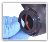
Outer silicone dust seals are placed directly against bearings. For added sealing, apply grease between seal and bearing.
