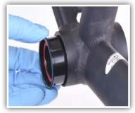
Insert drive side cup (female) into frame by hand.
