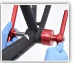
5. Spin on second handle and tighten handles together until you feel the bearing pop out of the cup.
