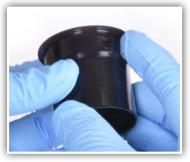
Apply a thin layer of high quality, carbon-safe grease or anti-seize compound to outside surface of each BB cup.
