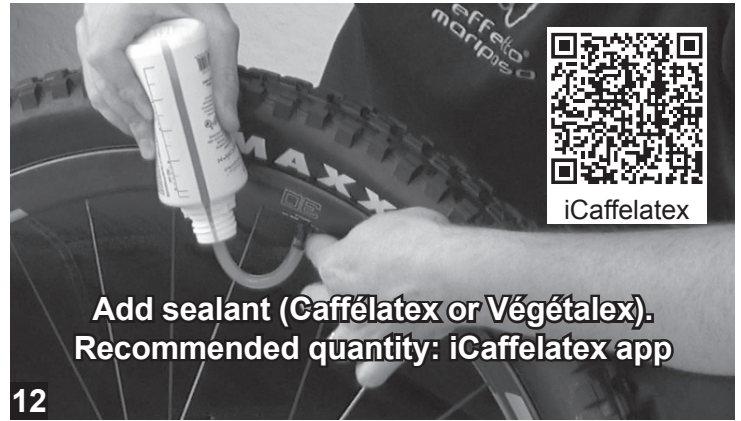
Shake/rotate tyre to spread sealant
