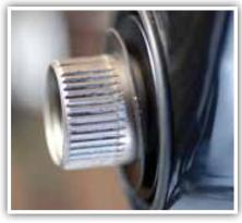
3. Take up any play in your cranks with our Crank Spindle Spacers. Place the spacers as shown in above illustration.
