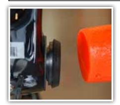
If not already installed, press PF30 bottom bracket cups into frame. Identify left and right side adapters. Start inserting adapters into bottom bracket bearings by hand. Seat adapters using a rubber mallet.
