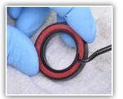
1. Lift up seal using a utility knife or pick. If servicing bearings outside of BB cups, remove both seals. Clean seals and set aside. For Angular Contact bearings, note which side takes the black seal.
