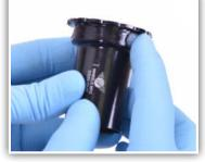
Apply a thin layer of high quality, carbon-safe grease or anti-seize compound to outside surface of each BB cup.
