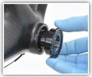
Insert non-drive side cup (male threads) by hand and turn clockwise until threads begin to engage. Do not cross-thread cups. Check that any internal wires or hoses are out of the way of the cup.
