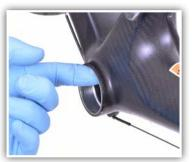
Thoroughly clean frame's bottom bracket shell. Do not install cups dry. Apply a thin layer of high quality, carbon-safe grease or anti-seize compound to inside surface of the shell.
