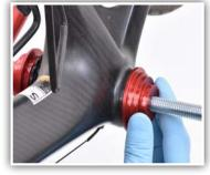
Slide second BB adapter onto threaded rod and into the opposite side of the bottom bracket shell. Match the correct step size with the BB shell inside diameter. Adapter should fit with little to no play.
