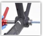
3. Insert handle, rod, pusher and adapter into the backside of the bearing you are removing.
