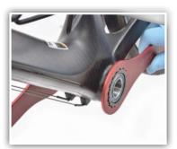
10. Frames with loose fitting cups may need a tool on each cup to fully tighten.
