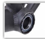
12. Remove press handles and adapters from cups. Bearing is now isntalled.
