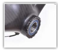
11. Bottom bracket is now installed. Install crankset per crank manufacturer's instructions.
