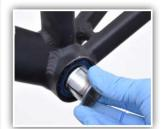
1. Insert appropriate size extractor into bearing. Push extractor completely in until you feel it snap in place.
