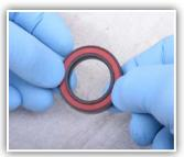
4. Lightly press seals onto bearing. Seals should sit flush to the outer face of the bearing races.
