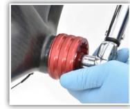
Continue to turn cup clockwise until flush against the outer face of frame. Finish tightenting cups using Wheels Mfg BB Socket [<u>BBT00L-48-44</u>] or Flat Wrench [<u>WRENCH-BB48-44</u>]. Tighten cups 35Nm - 50Nm.
