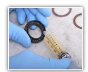
3. Pack bearing with new, clean bearing grease [<u>GR-001</u>].
