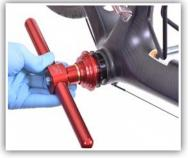
5. Using Wheels Mfg Universal Bottom Bracket Press [<u>PRESS-7</u> or <u>PRESS-7-PRO</u>], insert one BB adapter into drive side bearing. Match the correct size step on the drift with bearing inner diameter. Slide press handle + rod thru BB adapter and cup.
