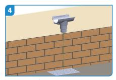
With the use of a plumb or laser line, position outlets over gullies and support with at least one bracket. Also include a bracket per angle (internal or external).
