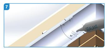
Trim 4-5 mm off top of nozzle so it fits snuggly into the large holes in the base of the union, inject the **special\* SnapIT Express** low modulus sealant supplied into one of the large holes in the bottom of the union until the sealant appears at both of the smaller holes at the rim of the union. Repeat the action on the other large hole. **(\*Sealant only available from us).**
