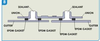
Ensure you apply the sealant gently to ensure the void is fully filled.
