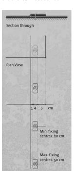
at least 80 mm. A nozzle width of 80 mm must therefore be used. The overlap between the upper edge of the membrane and the fastening plate is 50 mm. The distance between the lower edge of the membrane and fastening plate is 10 mm (with a total overlap of 100 mm) and 40 mm (with a total overlap of 130 mm). Both the distance and the total overlap can be larger if fastening plates with larger diameters or wider widths are used.
