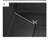
Make a mitre cut in the roof surface area situation. To comply with the overlap width, the diameter and the width of the formed parts / cut-outs must be at least 200 mm. The individual parts / cut-outs are fully surface-welded with hot air on the flashing strip with an overlap width of min. 40 mm. The seam connections of the individual parts / cutouts are also formed using hot air welding.
