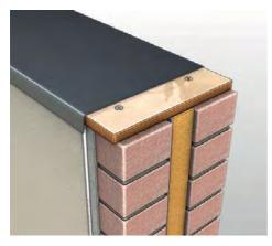
**1.** Ensure minimum 18mm marine ply and weatherproof membrane is fitted to the structure before commencing with the installation (all supplied by others).
