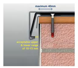
**3.** Secure brackets with minimum size No.12 x 50mm sized screws using the outer slots in the fixing straps at 1.5m maximum centres or as recommended based on wind uplift calculations or coping size. Additional screw fixings will be required on wider fixing straps. Maximum 40mm from fixing screw centre to external wall finishing surface.
