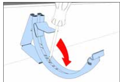
Use screwdriver to fold the tap forward for low inclinations and backwards for \alpha \geq 22^\circ .
