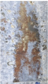
After 6 weeks salt spray test
