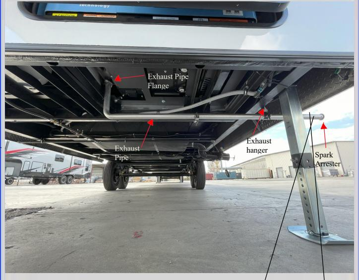
End of Exhaust Pipe must extend no less than 25.4 mm (1") beyond outer metal skirting or trim
