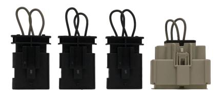
EACH BLACK CONNECTOR GETS PLUGGED INTO NOX SENSOR CONNECTIONS.
