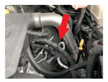
3. Install the NOx Sensor Plug on the passenger-side of the frame rail. This plug will be located on the frame rail behind the passenger door.
