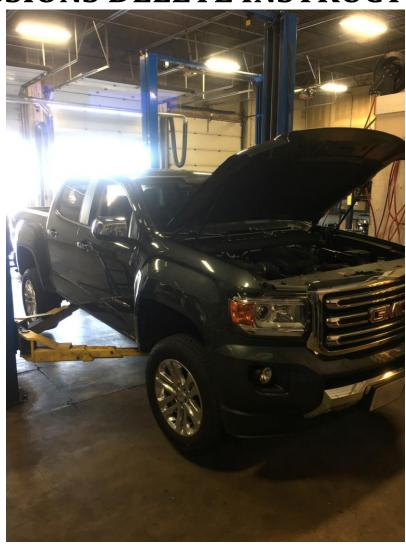
Drop the tray under the def tank (between spare tire and rear axel). Unplug def pump.
