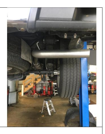
Install all clamps and tighten.
