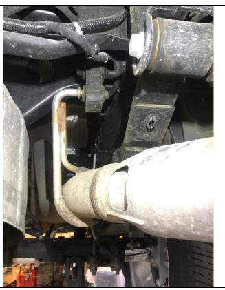
Remove exhaust from the two exhaust hangers in photo.
