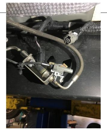
Remove exhaust fuel injector from exhaust pipe.
