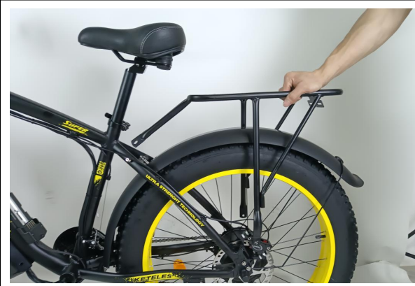
Fix rear fender and rear rack to the frame
