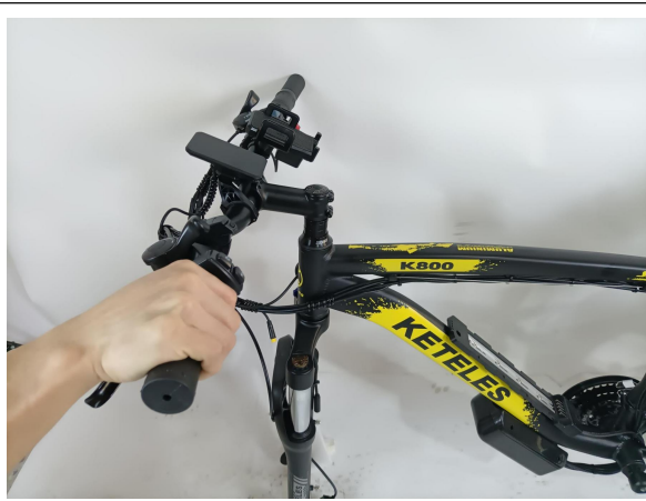
Fit the stem and handlebar together
