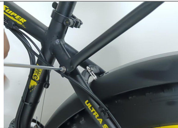
Tighten the two upper bolts on both sides
