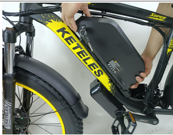
Push the battery downward and lock it
