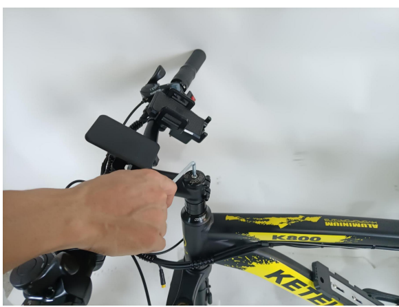
Tighten the bolts on the other side
