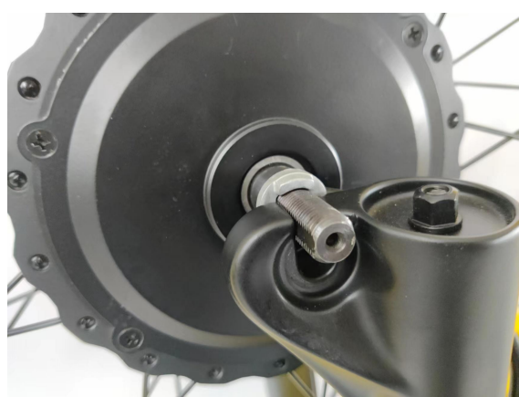
The axle of the motor goes into the grooves of the fork.
