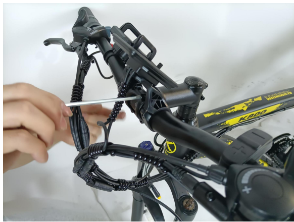
Tighten the 4 bolts that hold the handlebar
