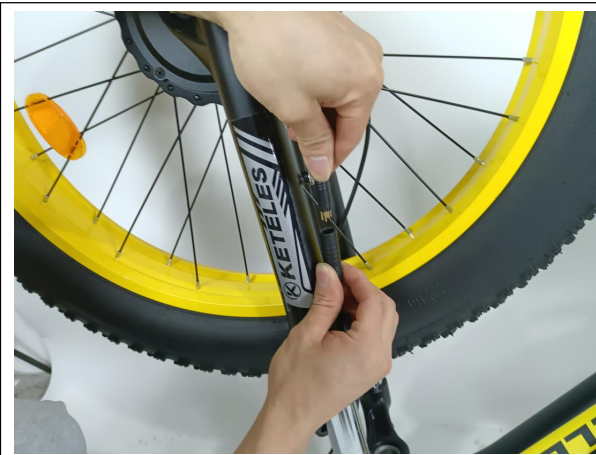
Connect the inline connectors of front motor cable
