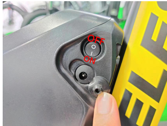
The charging port and the battery ON-OFF switch
