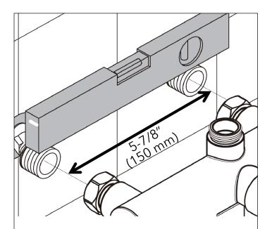
**3.** Adjust the adapters so they are level and exactly 5-7/8" (150 mm) apart on center.
