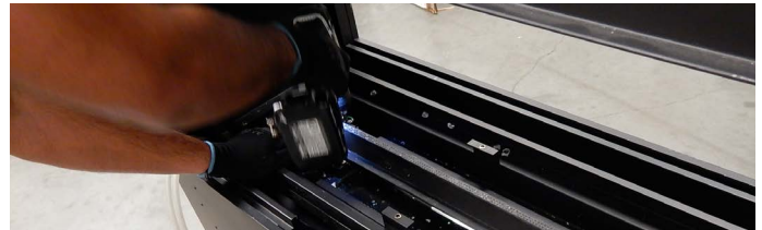
Figure 13. Removal of burner strip
