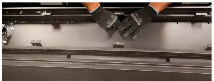
Figure 12.g Removing metal plate
