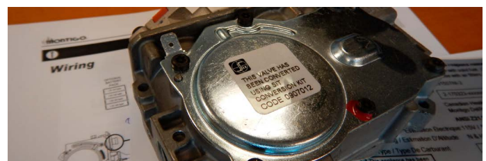
Figure 13.k Conversion label on valve
