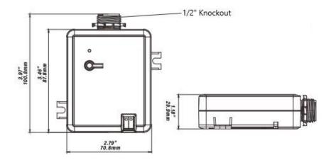
BLACK- 18 AWG AC INPUT 120V/277V WHITE- 18 AWG AC INPUT 120V/277V
