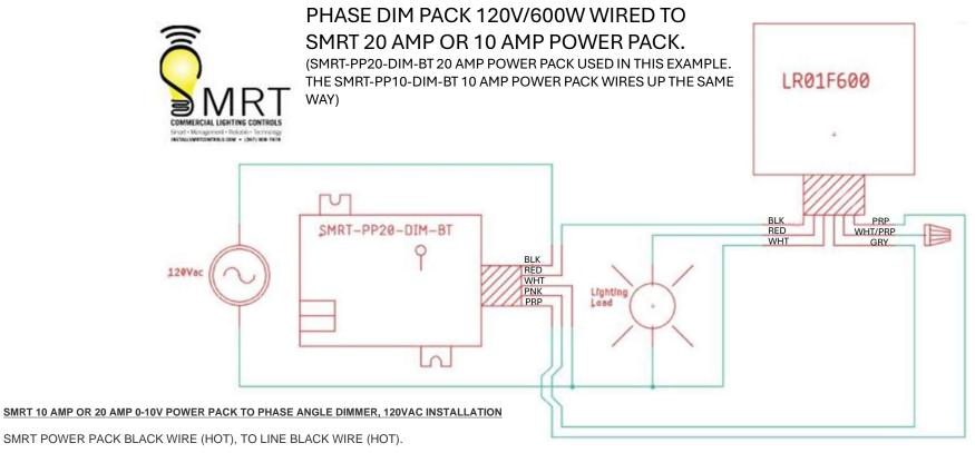
SMRT POWER PACK RED LOAD WIRE, TO PHASE ANGLE DIMMER BLACK WIRE (HOT).
