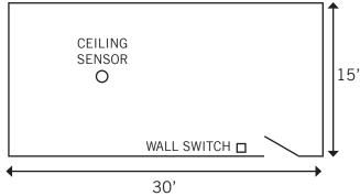
IN EXAMPLE 1, ONE KIT WILL BE ENOUGH FOR THE SPACE. ONE WALL SWITCH FOR 1 EXIT DOOR, ONE SENSOR WILL COVER THE SPACE, AND THE POWER PACK WILL CONTROL UP TO 1200 WATTS AT 120V, AND ONLY 560 WATTS ARE BEING USED.
