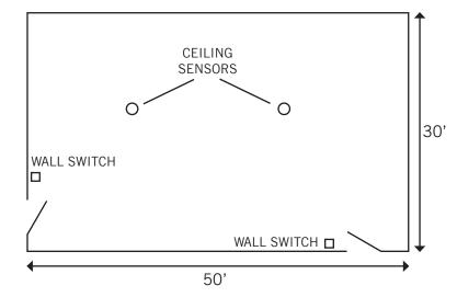
IN EXAMPLE 2, A LARGER SPACE, ONE KIT PLUS ONE ADDITIONAL SENSOR AND ONE ADDITIONAL WALL SWITCH IS NEEDED. THE POWER PACK IN THE KIT WILL CONTROL UP TO 2,770 WATTS AT 277V, AND ONLY 800 WATTS ARE BEING USED. ADDITIONAL SENSORS AND WALL SWITCHES CAN BE PURCHASED AT YOUR ELECTRICAL DISTRIBUTOR WHERE YOU PURCHASED YOUR CONTRACTOR PACK.
