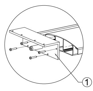
Remove the previous End Cap, use its screw to fasten End Cap, Angle Aluminum 1 and 2 to louver.
