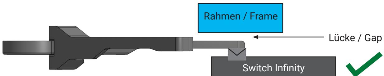
4. GGA-1 Adapter spannen / clamping of the adapter
