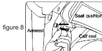
Figure: hex head screw fixed in front part of armrest
