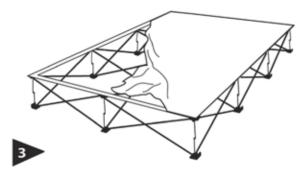
Work in continuous direction around the frame until graphic is completely attached.
