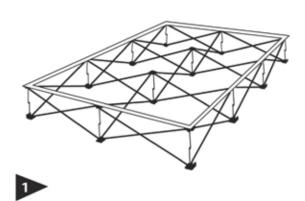
Assemble frame and lay flat on its back. Remove existing graphic.
