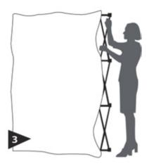
Lock all hooks between front and back hubs.
