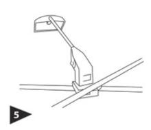
**OPTIONAL** Attach lights to top of frame by sliding the plastic X Blocks under the frames cross sections.
