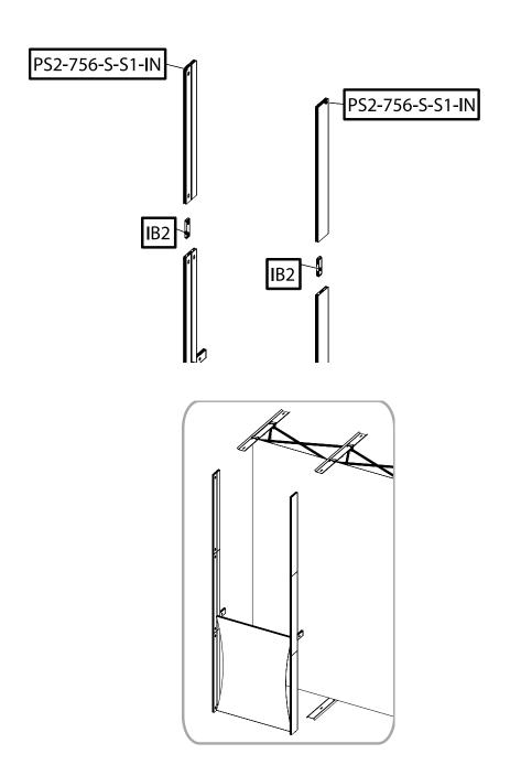
Lock extrusion frame onto top and bottom stabilizing feet, using fixed cam lock. With Allen Key tool, turn one quarter turn to lock into place.
