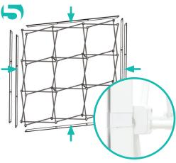
Attach channel bars to frame. Slide channels bars onto frame, from top to bottom, then secure onto metal peg.
