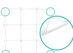
• Connect the top and bottom End Caps on each side of the frame.
