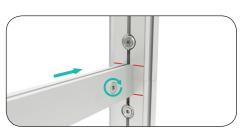
**b.** Align Support Struts within marked lines, and insert End Lock into top and bottom grooves of frame.
