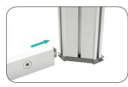
**c.** Connect horizontal extrusion to the bottom of a vertical extrusion, screw facing inward.
