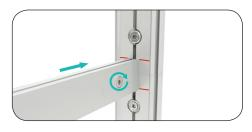
**b.** Align Support Struts within marked lines, and insert End Lock into top and bottom grooves of frame.
