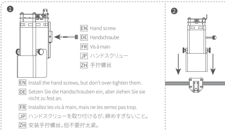
EN Attach the laser module to the x-axis integration part and tighten the hand screws (loosen the hand screws to adjust the laser module up or down).
