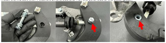
**Step 7:**Install the M8 mounting bolt and M8 locknut. Do not over tighten the bolt, it just needs to be snug to the pedal.
