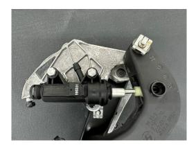
**Step 3:**Sand down any raised castings that prevent flush installation. You just need to remove any raised imperfections from the casting process. Don't overdo it and remove too much material.
