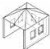
Figure 5 - Open side at least 25% of total wall area. 30 percent or more in total of the remaining wall area is open and unrestricted.
