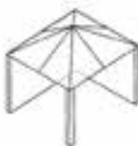
Figure 2 - Partial Enclosure with overhead cover and no more than two walls.
