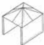
Figure 3 - Partial Enclosure with overhead cover and no more than two walls.
