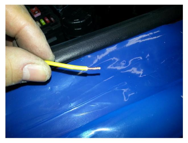
Locate the 5 amp fuse in the fuse box and add this fuse circuit and plug yellow line into this circuit – add additional 5 amp fuse:
