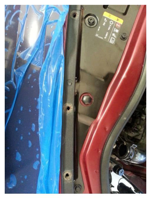
Remove the push pins and bolts that hold the upper part in place:
