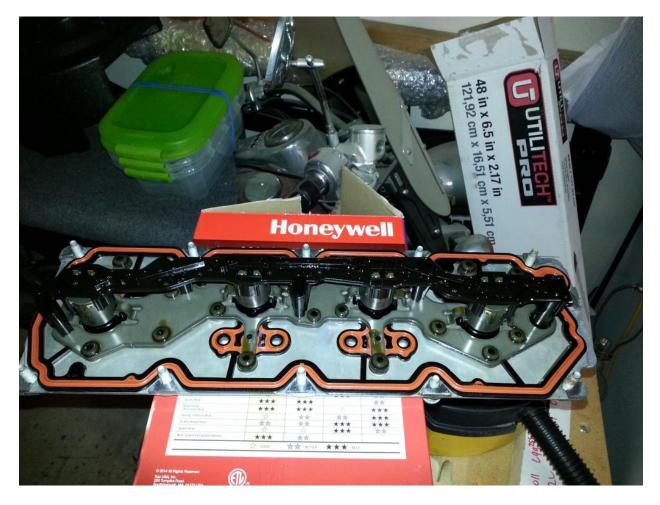
New valley cover with oil sending unit installed and bolted:
