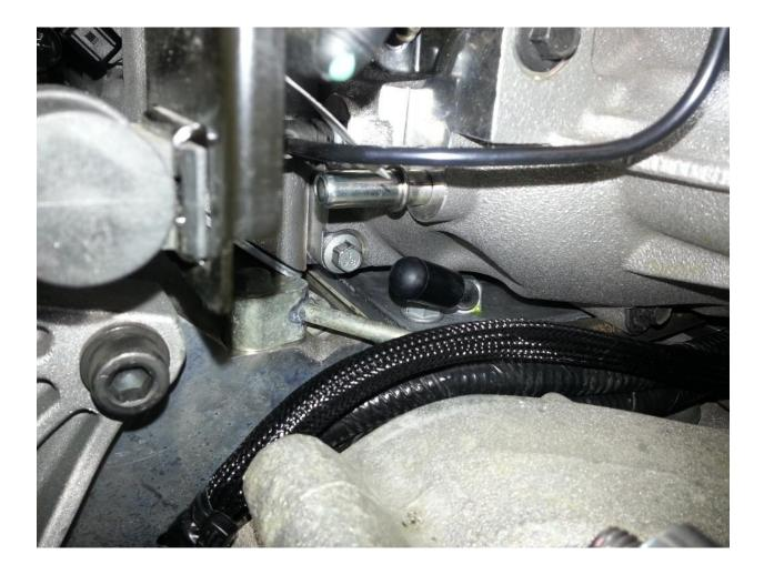
Open the covered Supercharger intake, then install all 10 bolts (used blue loc-tite) use a 'magnetic' 10mm socket to prevent any 'accidental' dropage:
