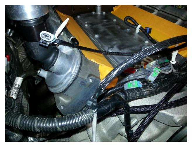
Now, with the wiring done, now is the time to install the new Tensioner and pulley assembly. You will need to remove 1 bolt from the water pump (passenger side) – this will not be reused:
