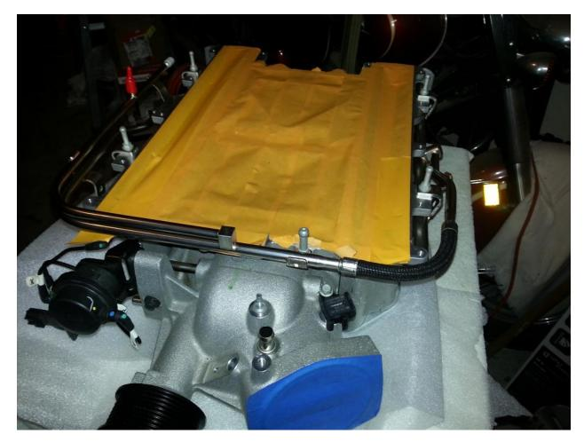
□ Now is the time to wire up the MAP, Throttle Body, and EVAP sensor connectors.
