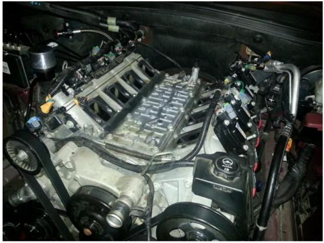
□ Once the intake is off, sweep and then clean the intake openings and tape them – don't allow dirt to fall into the intake openings:
