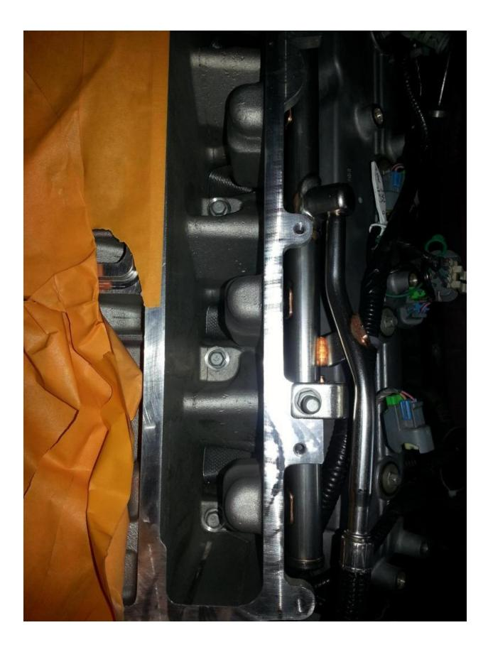
Plug in oil pressure sensor before you torque the intake:
