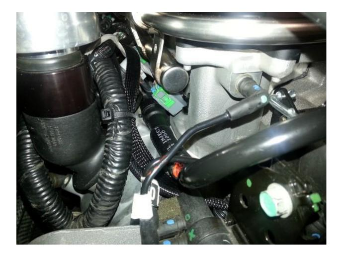
□ Install hoses as necessary (upper radiator, steam, lower) make sure all connectors and hoses are clear of the pulleys:
