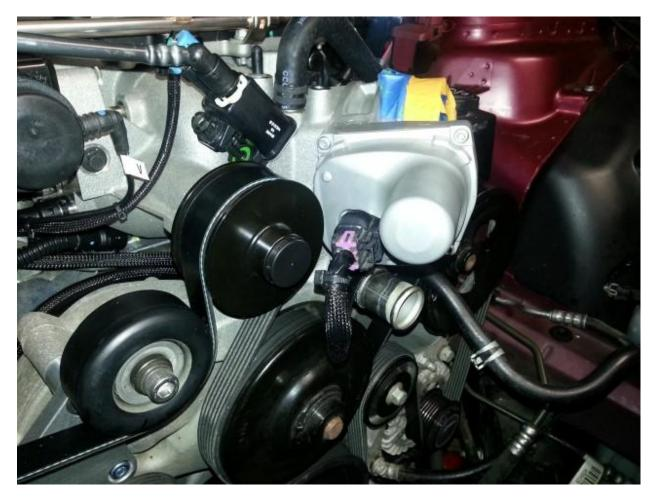
Connect the throttle body connector – make sure to route and avoid all pulleys:
