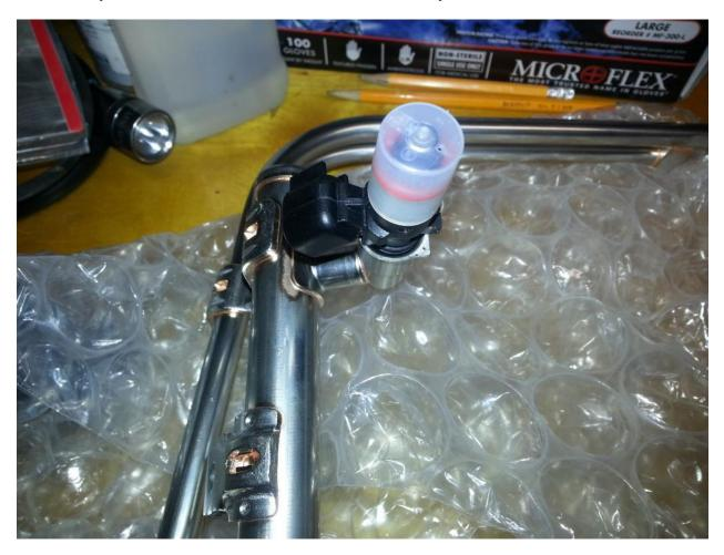
Place each injector in its location – note the orientation of the injector:
