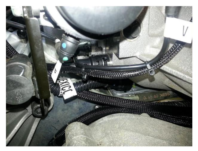
Verify all wires are clear of obstructions and all vacuum lines and PCV lines are hooked up:
