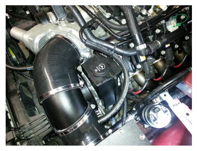
□ Now is the time to review and verify all vacuum lines, connectors, fuel lines, belts, spark plugs and wires, coil packs, and hoses are connected. Verify NO leaks. It is best to re-install the front wheels, place the car on the ground, and use tire blocks before starting.
