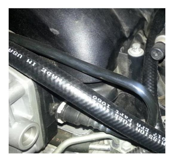
□ Remove the EVAP line and connector (marking the connector as you'll need to extend the wire) from the EVAP solenoid:
