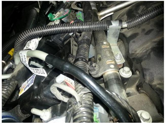
Remove fuel line from hard line near passenger side (use a shop towel to trap any spillage and use all safety precautions). You will not be reusing the hose, but will reuse the clips so save them aside. Cover the open fuel hard-line to prevent any fuel from leaking:
