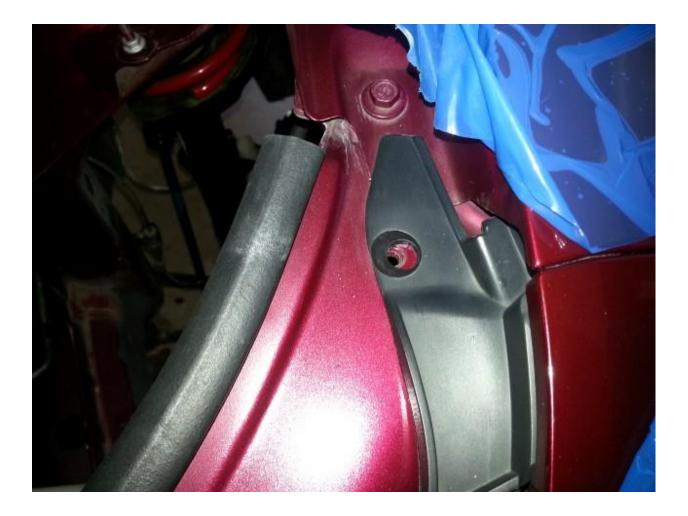
Protect the lower portion of the bumper, and pull the bumper forward and off the car (watch for plastic spacers along the top ridge of the bumper):
