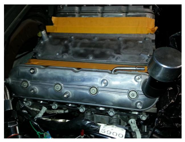
Valley cover bolts are torque to 18 ft. lbs., oil sender is 15 ft. lbs.
