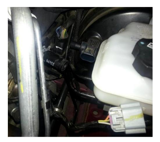
The L99 has a brake booster connector that you will also need to remove and mark the connector for reassembly. The booster hose from the manifold is NOT re-used. □ With all the intake bolts loosened all the way, the fuel lines removed, vacuum hoses removed, injector connectors removed, lift the intake and set aside. Be careful and do not let dirt fall into the opening of the head:
