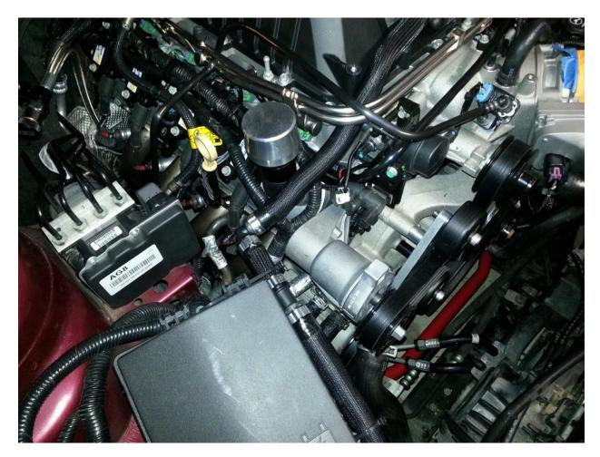
Tighten all hose clamps. Fill reservoir with 50/50 Dexcool. It will be necessary to 'milk' the lines to get the fluid through.
