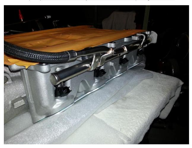
Installation requires you do the 'drivers' side injectors first to allow for the passenger's side to fit:
