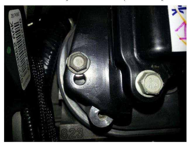
Note the bolt is 'raised' from the original location. You'll need to drill just above the existing hole:
