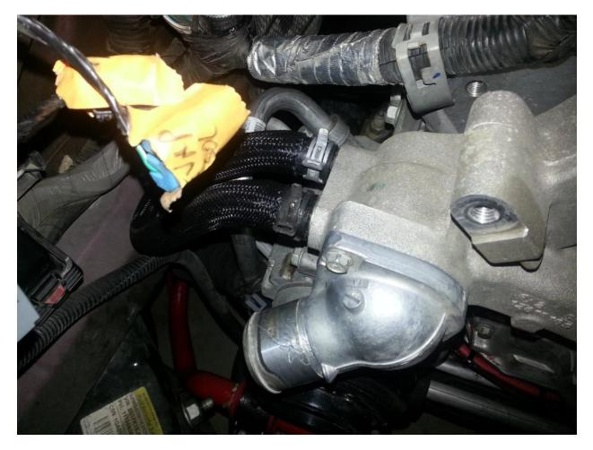
□ Relocate the ground from the 'front' of the head to the location on the 'passenger's' side of the head (it will be necessary to shorten the bolt – using a nut and a hacksaw, trim the bolt length by about 3 to 4 threads):
