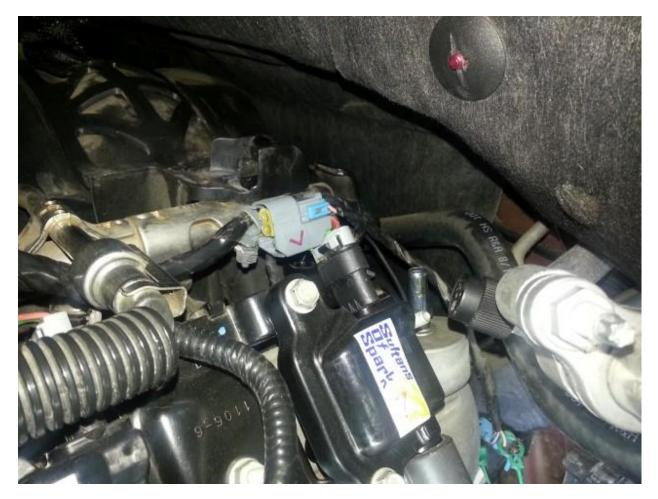
Note that each connector should be marked to assist in re-assembly later.
