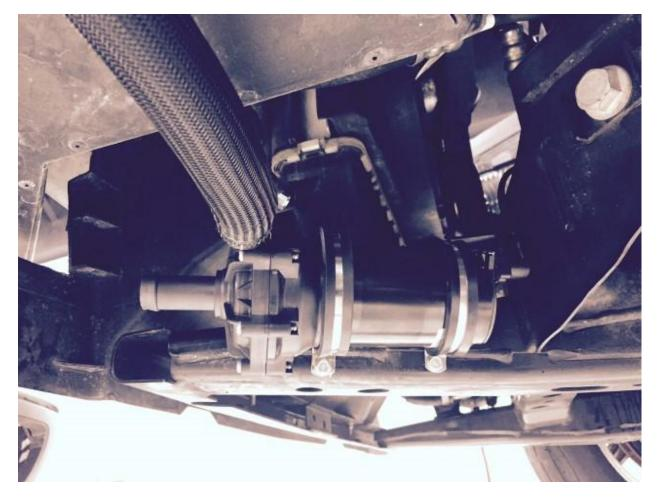
You can now route the hose from the pump to the inlet of the Heat exchanger (flow out is from the side):
