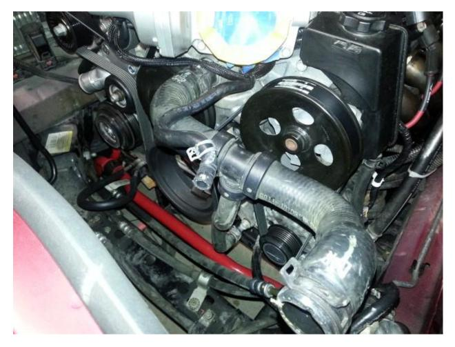
□ Prepare heat exchanger install. The front of the car will need to be removed. It is best to raise the vehicle, remove the front wheels, and remove the splash shields. This will give you access to the front bumper bolts:
