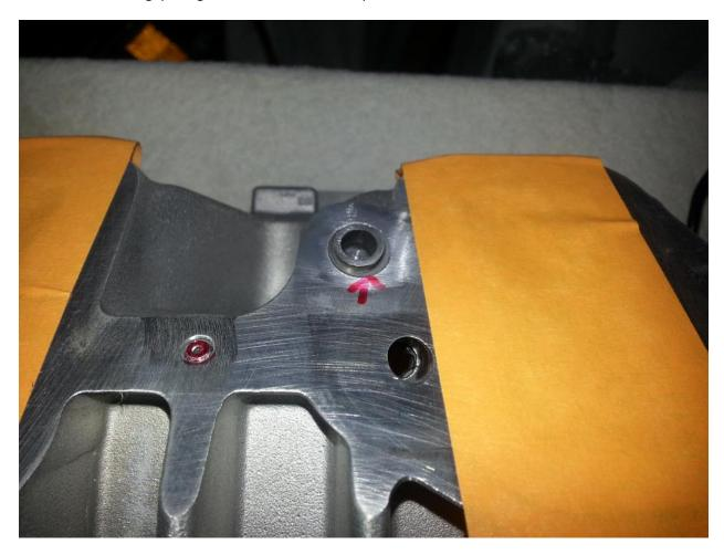
□ If necessary, remove any 'existing' rivets from the manifold:
