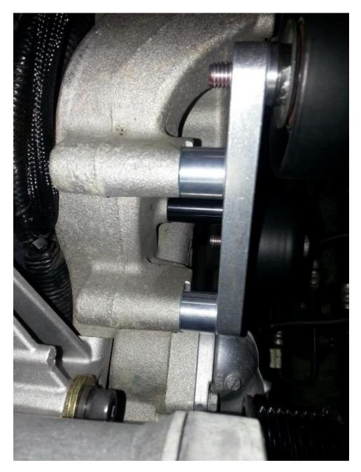
The two bolts main bolts (use RED loctite) on the top are torque to 32 ft. lbs. The 'water pump' bolt is torque to 19 ft. lbs. USE BLUE loctite on the water pump bolt.
