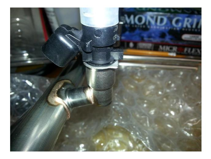
All injectors installed – awaiting clips:
