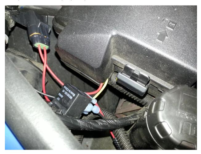
Tie-wrap the harness' and verify they don't pinch when the fuse box is closed:
