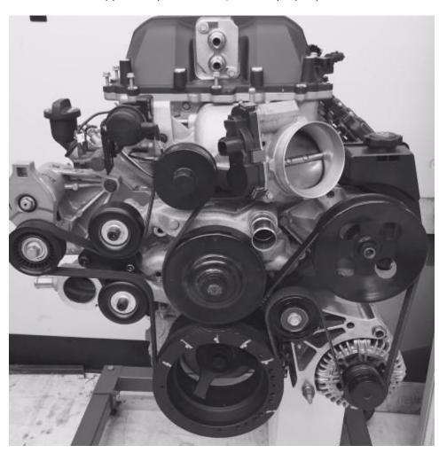
□ Install the kit supplied serpentine belt (note the proper position on the tensioner):
