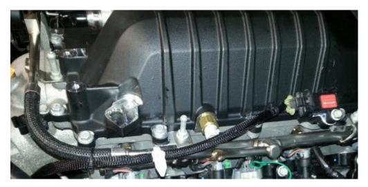
□ Install the brake booster hose (and connector if required), vacuum hoses to the manifold:
