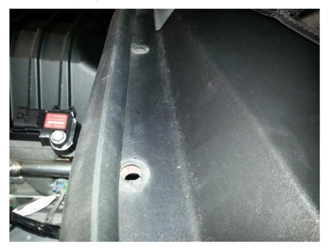
□ Using these types of tools, begin bolting down the lib (follow this sequence): To bolt down the # 15 and 16 bolts, you'll need to use a hammer handle (after you've tighted bolts 1-14) to give you better access:
