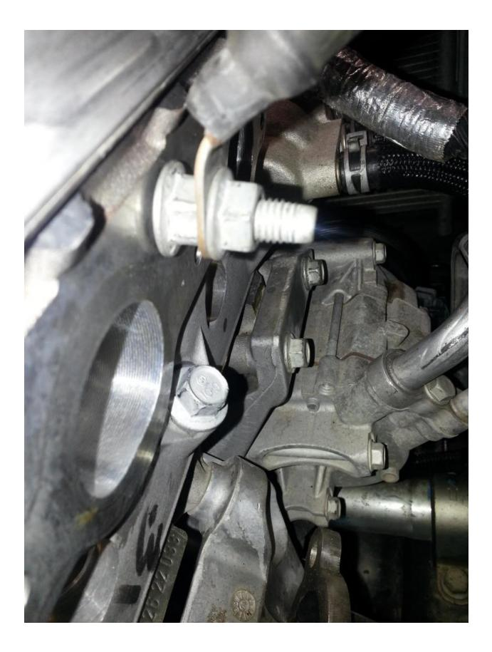
□ While the coils are off, this would be the right time to install the new Spark plugs. These should be the correct 'range' for running the supercharger (8 total) NOTE: these do NOT require anti-seize. Torque to 15 ft lbs:
