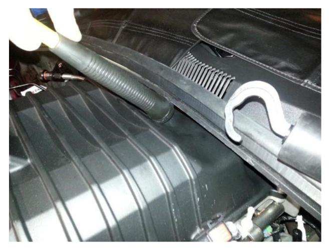
Reinstall the previously removed push pins back into the cowling.
