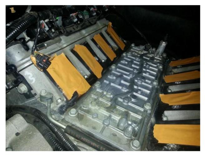
You can also remove the throttle-body from the intake if you have not done so – you will reuse this on the supercharger.
