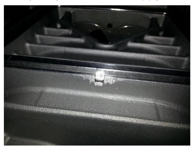
□ Install 'orange' intercooler gasket into lower manifold – note orientation of proper gasket installation:
