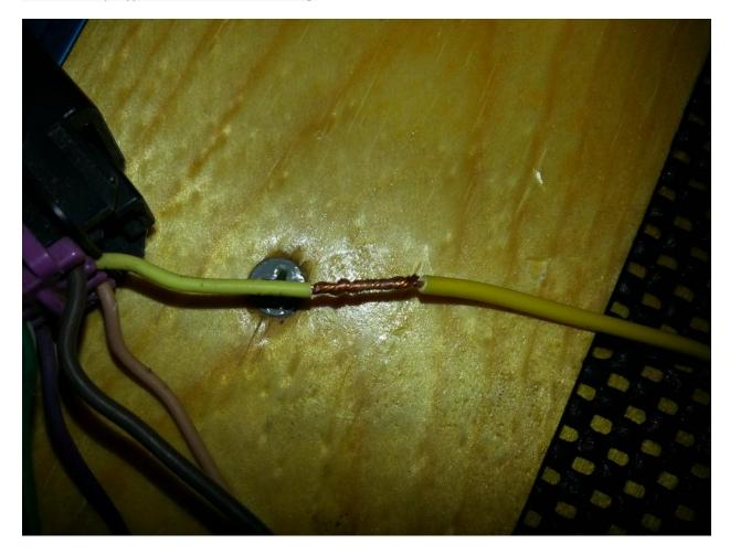
This is a 'wrap' type connection for soldering:
