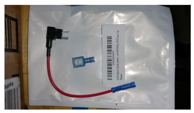
Connector for yellow wire and add a circuit (for the 5 amp fuse):
