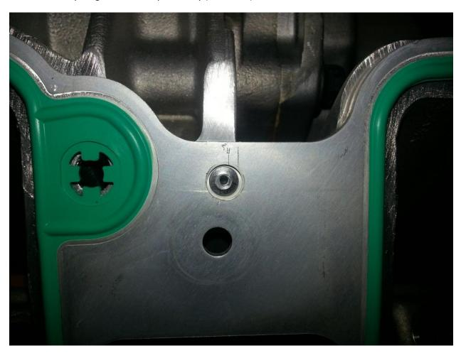
Make sure everything is centered up correctly (bolt holes) and rivet the NON-ELONGATED rivet first:
