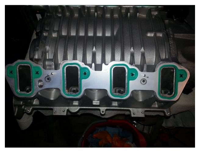
Place the rivets in the gaskets and set on manifold:
