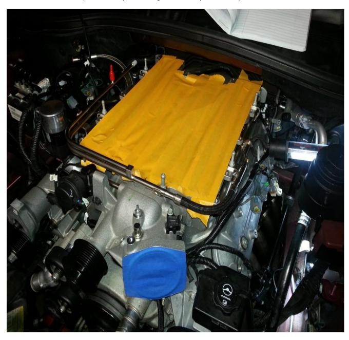
With the intake bolts torqued, cover up so nothing falls in until you are ready for the lid:
