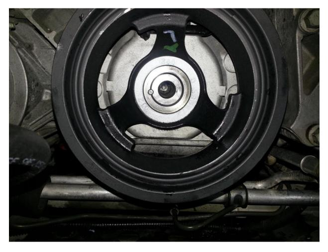
Bolted per pinning instructions (use red loctite on bolt threads) each car is different so verify the steps the proper torque steps and sequence:
