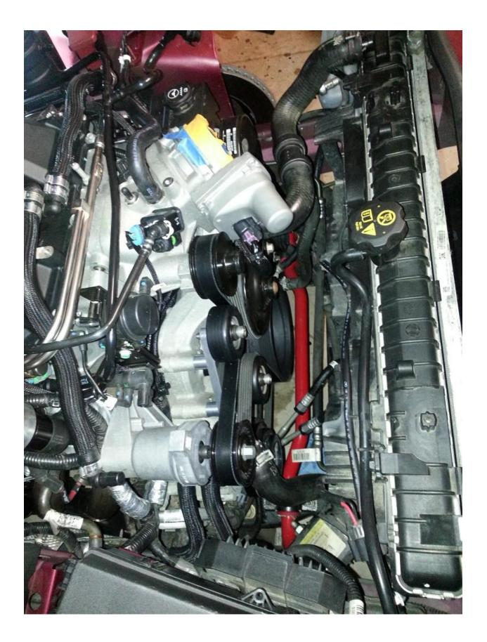
□ Install the PCV line from the valley cover to the super charger lower manifold:
