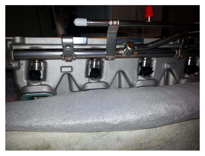
Bolted down -- NOTE leave OFF the very front bold on the fuel rail – you will have issues with removing the fuel rail should you need to while the 'lid' is on (the picture does show it on, but it was ONLY for show):
