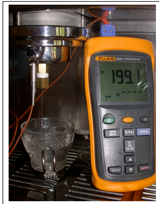
Fig. 3 Installed portafilter thermometer measuring the temperature of the metered brew water stream.
