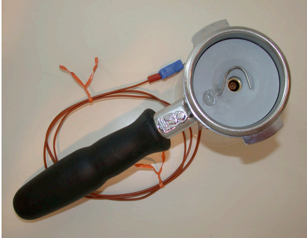
Fig. 1 Portafilter thermometer top view, showing the Type T thermocouple probe and the coffee cake facsimile.
