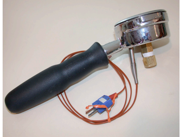
Fig. 2 Portafilter thermometer side view, showing the thermocouple probe's exit through the bottom of the portafilter, and the brew water metering orifice.
