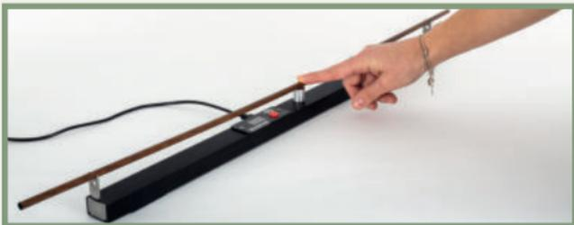
Bend the arrow by pushing it straight down to the centered block and hold until spine is determined.
