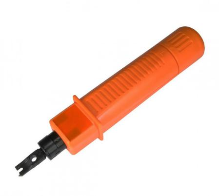
4XEM's professional grade impact punchdown tool is the perfect multi-purpose tool for punching down Cat6a/Cat6/Cat5e/Cat5 cable to 110-Type jacks and patch panels or telephone wire to 66M blocks. Both blades (110 & 66) have cutting and non-cutting sides. Built to perform, this tool features a ridged alloy steel frame with a storage compartment in the body for the blade not in use.
