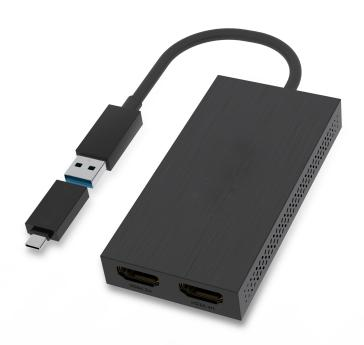
The USB 3.0 to Dual HDMI 4K Display Adapter is a high-performance solution for anyone looking to expand their display capabilities. With its USB 3.0 Type-A Male (5Gbps) host connector, this adapter makes it easy to connect two HDMI displays to your computer, laptop, or other device. The dual HDMI 1.4 Female (10.8Gbps) ports offer stunning 4K resolution, allowing you to enjoy sharp, clear images and video on two monitors.
