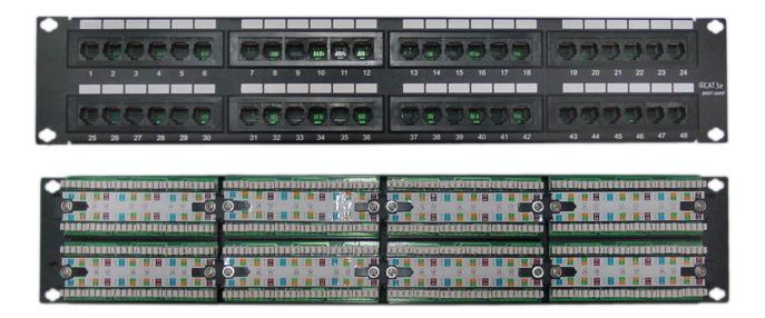
4XEM's Category 5E Patch Panels offer 110-type termination while meeting and exceeding EIA/TIA TSB-40 Cat5E connecting hardware specifications. Color coded for both EIA/TIA 568A & 568B installations. 24 ports with 50µ gold-plated contacts ensure quality connections and a wide range of plug and play options. Clear numbering on both the front and back of each panel provides a quick and easy way to identify cable runs.
