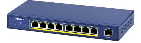
With Power over Ethernet (PoE) available on all 8 ports, 4XEM'S 8-Port PoE 10/100M Desktop Switch (4XLS5008P) delivers fast 10/100Mbps Ethernet network capabilities plus industry-standard IEEE 802.3af power over UTP Cat 5 or higher to network devices such as IP telephones or surveillance cameras. Works right out of the box, with no software to configure. A simple, cost-effective, and highly reliable network data connection, it makes a great solution for expanding your home or office network.
