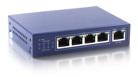
With Power over Ethernet (PoE) available on all 4 ports, 4XEM'S 4-Port PoE 10/100M Desktop Switch (4XLS5004P) delivers fast 10/100Mbps Ethernet network capabilities plus industry-standard IEEE 802.3af power over UTP Cat 5 or higher to network devices such as IP telephones or surveillance cameras. Works right out of the box, with no software to configure. A simple, cost-effective, and highly reliable network data connection, it makes a great solution for expanding your home or office network.
