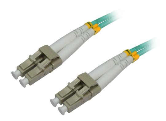
Laser optimized for reliability and blazingly fast 10 Gbps performance, 4XEM's Multimode 50/125um Duplex Fiber Patch Cables provide almost three times the bandwidth of 62.5um multimode fiber. Each end sports high quality, pull proof LC connectors with 1.25mm zirconia ferrules. Wrapped in a durable PVC jacket, every cable is tested for insertion loss before shipment and inspected to ensure GR-326 requirements are met.
