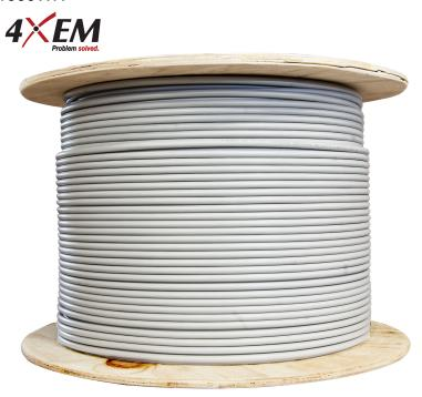
4XEM CAT6A is ideal for high-end solutions such as 10 Gbit Ethernet, and broadband video. This Cable consists of eight solid 23AWG wires and a separator to separate four pairs. CAT6A is also capable of great data transfer speeds than a CAT6 allowing greater improvements to any network. Included in package: 1000 ft Roll of CAT6A Cable 23AWG, 0.5mm HDPE (High-density polyethylene) jacket material in a White finish
