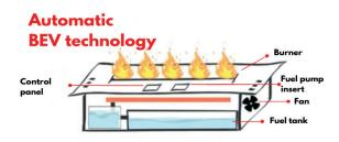
Automatic BEV technology guarantees the complete separation of fuel tank and fire line. This, coupled with multiple sesors, meets even the most robust safety requirements.
