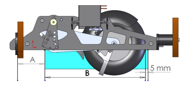
Dimension B at the end of the wheel plus 5 mm gives the length of the flap shaft. We cannot give this as a general rule here, as the landing gear is manufactured individually and has wheel legs of different lengths (FES).
