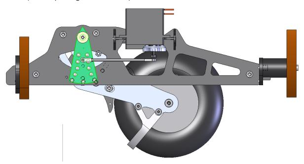
To check this position, even when installed, a mark has been made on the side panel which should be flush with the tip of the CFRP actuating lever (areas marked in red here). For this purpose a piece of wire can be placed on both side parts.
