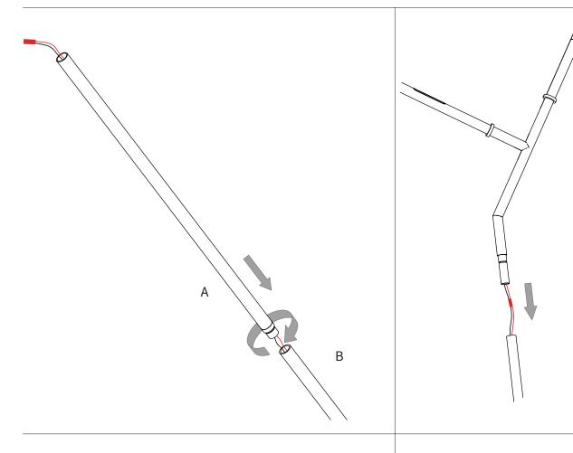
1 - JOIN THE TWO PART OF THE ROD. SCREWING THE PART A WITH PART B.
