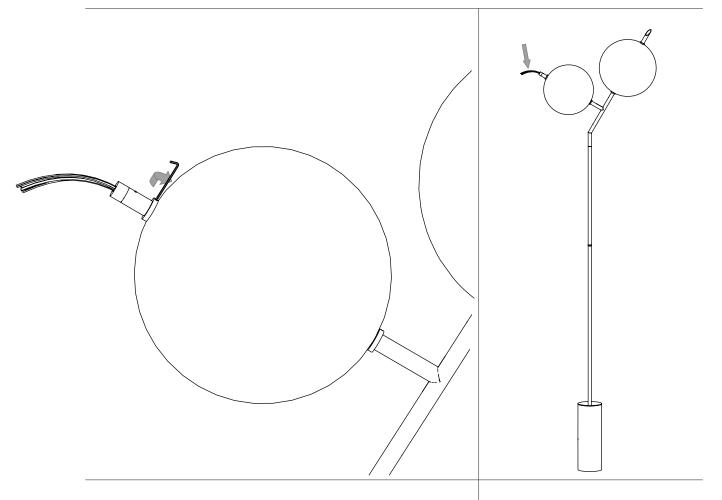
9 - BLOCK THE RING IN POSITION USING THE PROVIDED ALLEN-KEY. DO THE SAME FOR EACH RING.
