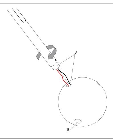
1 - GENTLY SCREW EACH ROD ONTO THE CORRESPONDENT HOLE ONTO THE SPHERE.
