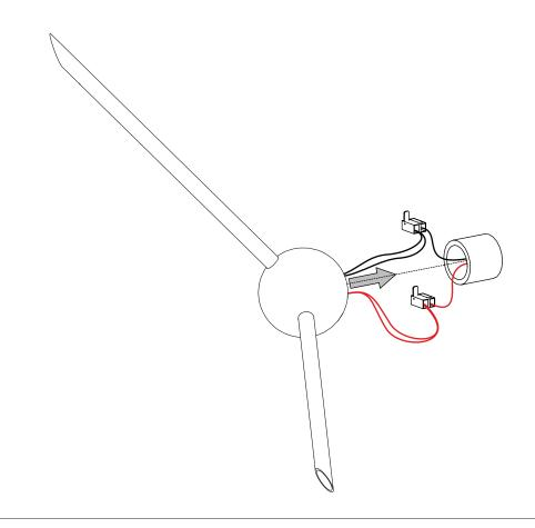
3 - MAKE ELECTRICAL CONNECTIONS PAYING ATTENTION TO THE POLARITY. (RED +24Vcc) JOIN THE TWO RED WIRES AND CONNECT AT THE WIRE NUT. DO THE SAME WITH THE BLACKS.
