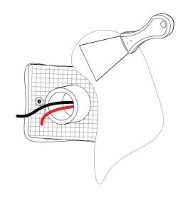
${\tt 1B}$  - CONNECT THE N-L INPUT OF THE TRANSFORMER TO THE ELECTRICAL SYSTEM AND PLACE IT INTO THE JUNCTION BOX.
