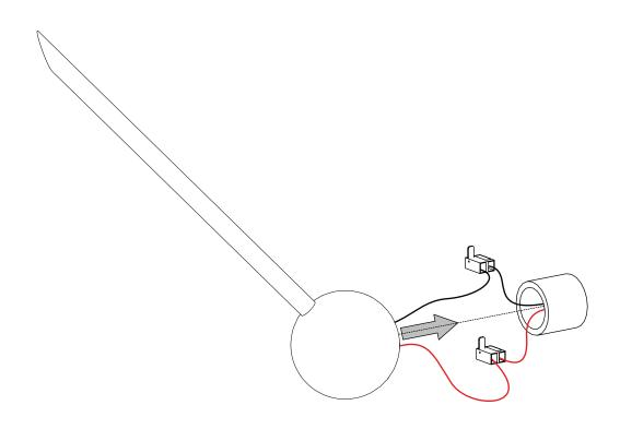
3 - MAKE ELECTRICAL CONNECTIONS PAYING ATTENTION TO THE POLARITY. (RED +24Vcc) JOIN THE TWO RED WIRES AND CONNECT AT THE WIRE NUT. DO THE SAME WITH THE BLACKS.
