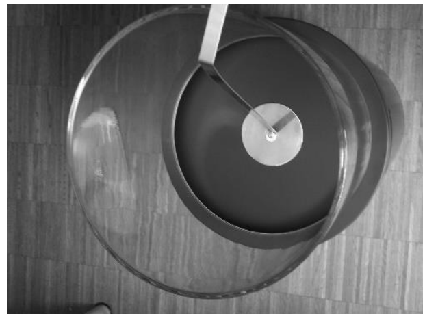
Fig. 2 : Closed Burner, the shovel covers the opening.
