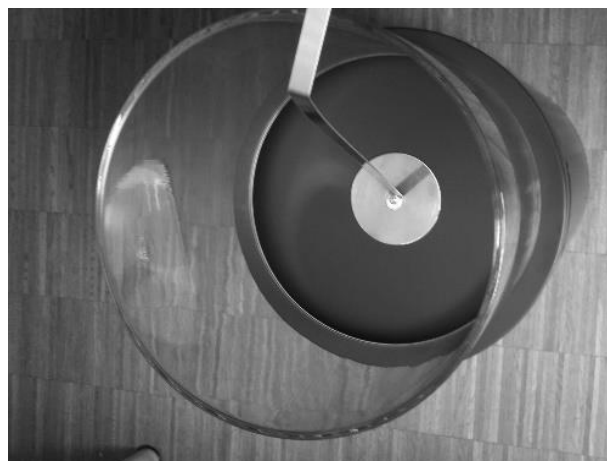
Fig. 2 : Closed Burner, the shovel covers the opening.
