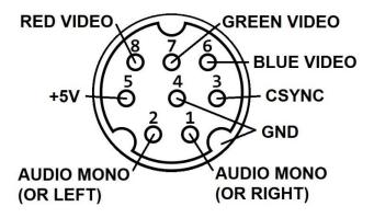
**Side note:** The connector has the same pinout as the XRGB mini and you can connect the HAS to the XRGB mini using an 8pin mini DIN cable. Pins of the cable must connect straight through end to end (1:1). When you connect the cable to the 3.5mm audio jack connector, it will override the audio that goes through the 8pin mini DIN.
